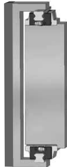
(8) Symmetrical assembly of the top and bottom of block, rail transfer
